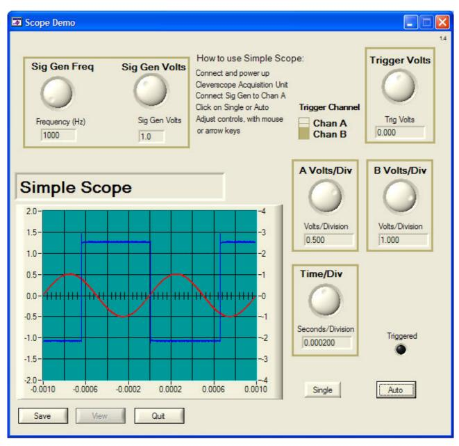
You can see there are controls to set the time base, the A and B channel gains, the trigger channel and amplitude, and the signal generator frequency and amplitude. As such it represents a simple example for use of the major features of the Cleverscope Acquisition Unit.
